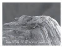
(a) 积屑瘤和沟槽磨损形貌
